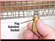
Loosen then remove the Fog Solution Socket. This will free the Protective Wire Guard.
