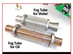
Side-by-Side comparison of the different Fog Tubes. Shorter Water tube has a flared end.
