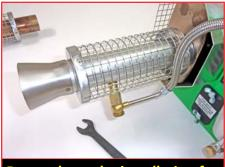
Run and test the installation for leaks. If a connection leaks, use a wrench to snug tight.
