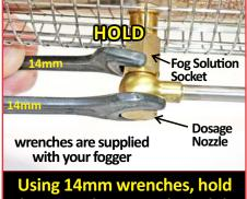
Using 14mm wrenches, hold the Fog Solution Socket while removing the Dosage Nozzle.
